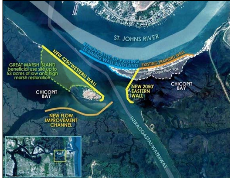
Figure 1. USACE design of the Flow Improvement Channel
